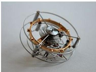
An assembled tourbillon, clearly showing balance wheel, pallet fork and escape wheel.
